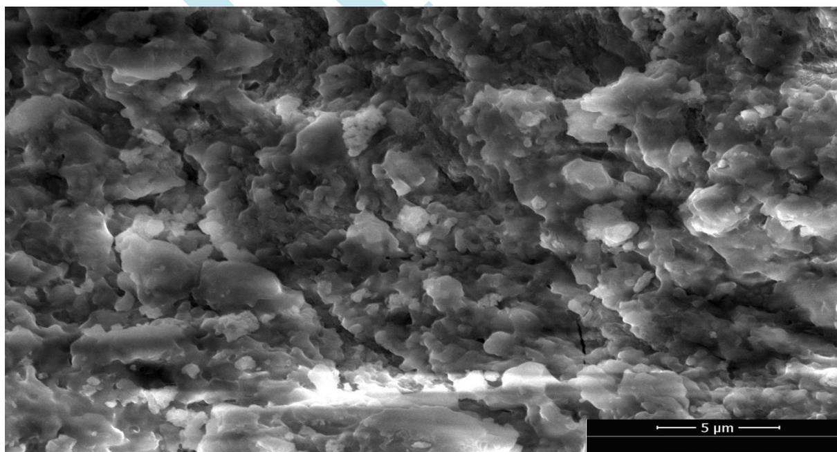
Fig. 6:- SEM images of Mg doped Zn Nanoparticles
