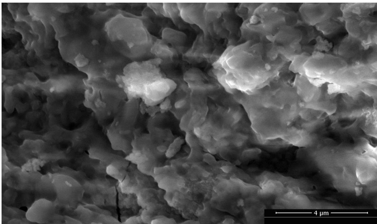
Fig. 7:- SEM images of Mg doped Zn Nanoparticles
